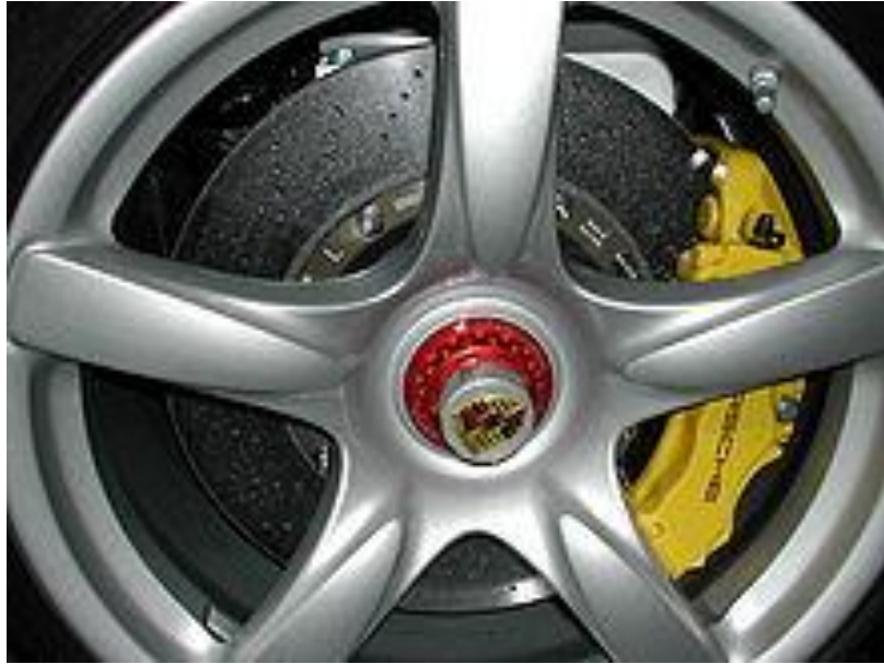
The Porsche Carrera GT's carbon-ceramic (SiC) composite disc brake
