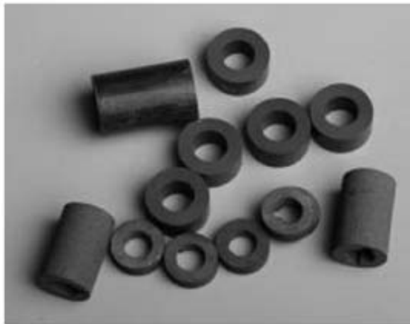
Ring shaped CIM Mn-Zn ferrite samples (outer diameter d_o=15\text{mm} , inner diameter d_i=6\text{mm} , thickness t=5\text{mm} ).
