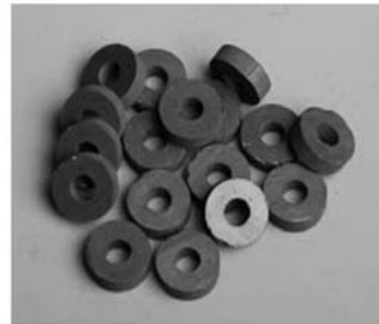
Ring shaped CIM Mn-Zn ferrite samples (outer diameter d_o=15\text{mm} , inner diameter d_i=6\text{mm} , thickness t=5\text{mm} ).
